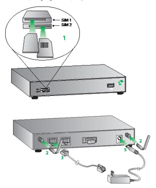
**Step 1) (SIM card models only) - Install the SIM card(s):** SIM card(s) should be inserted into SIM Sockets as illustrated in the above Front View image. For SIM 1, the contacts should be face down. For SIM 2, the contacts should be face up. In both cases, the end of the SIM card with the chamfered corner should be inserted first.
